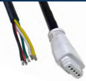
Male AURRO STYLE Connector to Bare Wire Item #4300-AURRO-5PIN-M-FC Voltage: 24V Max Amps: 10A Length: 8" (200mm) IP: IP67 Rated
